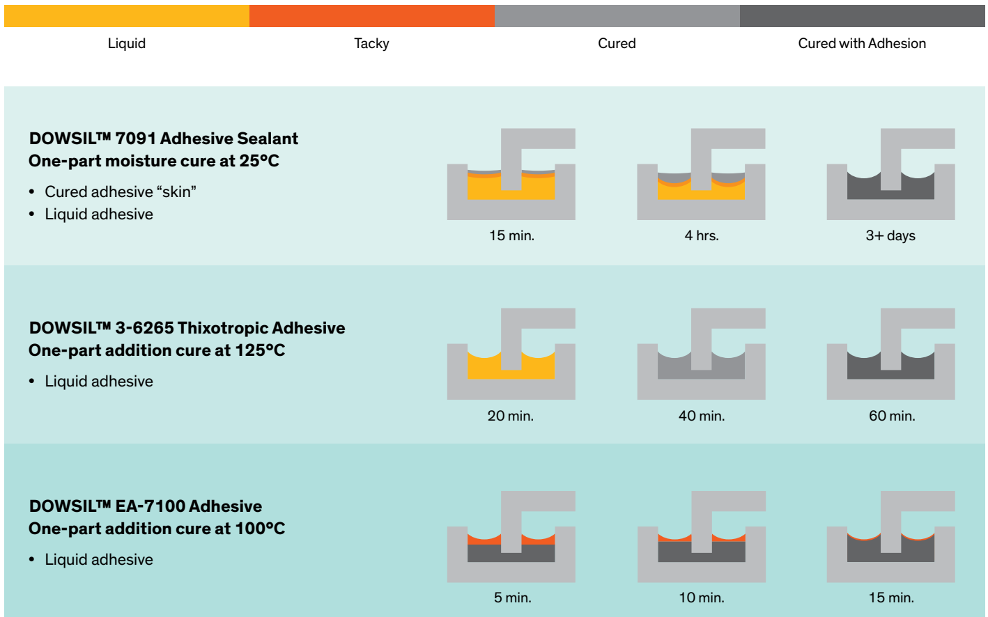
Figure 4: Cure comparison in a typical lid seal design in oxygen environment
